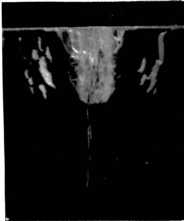
Plate I. Unconfined .5-inch long 10-grain MDF detonated on .5-inch Plexiglas Plate.
